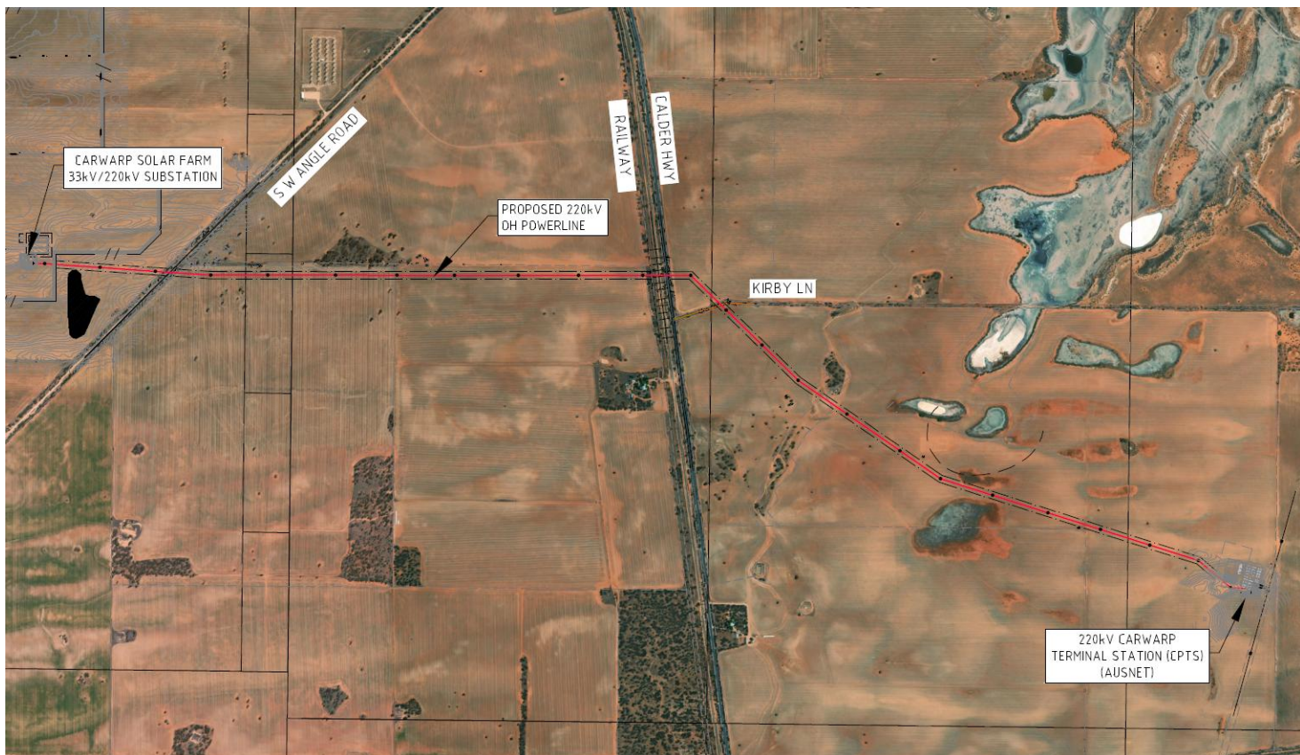
Figure 1 Overall route plan – 220kV OHTL
